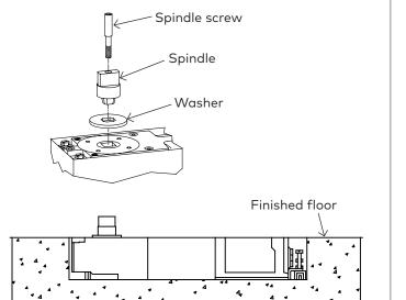
NOTE: Top of cement case must be flush with finished floor.
